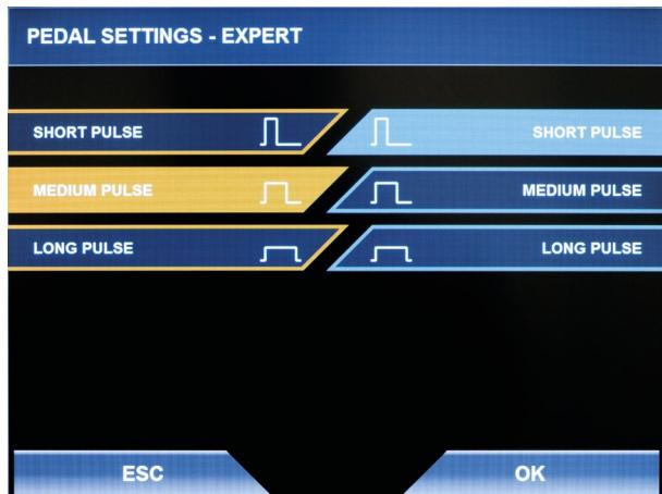
**MegaPulse 70+** offers experienced users the option to select the pulse width in three stages – short, middle and long. This covers a broad spectrum of 50 µs – 1100 µs.
