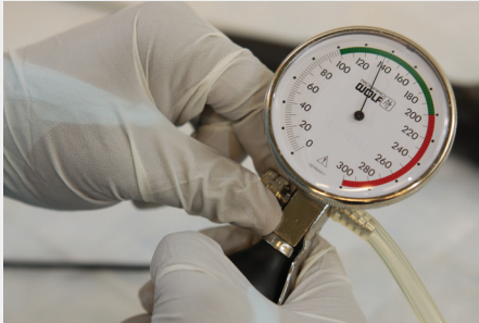
Inspect and perform leakage test
